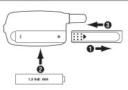
The LCD remote control is powered by a 1.5 Volt AAA Alkaline battery. When the power of the battery weakens the battery icon will be displayed on the screen. When the old battery is replaced with a new one, there will be a beep to indicate the power is up. To replace the battery, follow the steps in the illustration at left.
